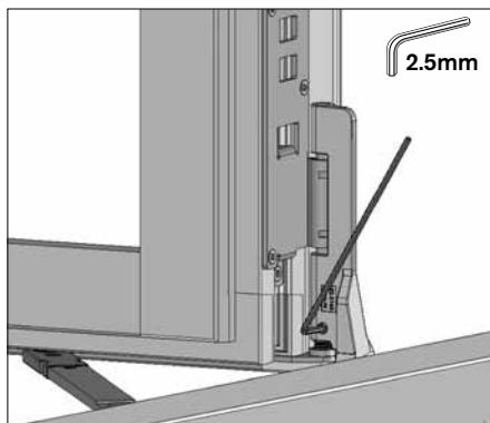
► **Height adjusting in the bottom hinge.** Open the window to maximum position. First loosen the set screw placed horizontally at the hinge.
