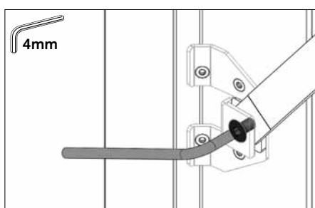
► **Adjusting the friction arm:** Loosen or tighten the screw. Adjust equally tight on both sides. **N.B.** Do not oil!
