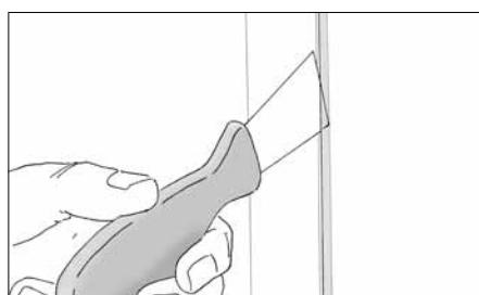
► **Carefully slip a putty knife between the frame and the backboard seal.**
