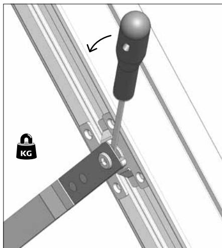
► **Dismounting:** Open the window to maximum position. Support the sash and dismount the balance arms using a screwdriver to unclick the balance arm on both sides of the sash. Turn the balance arm downward after disassembly.
