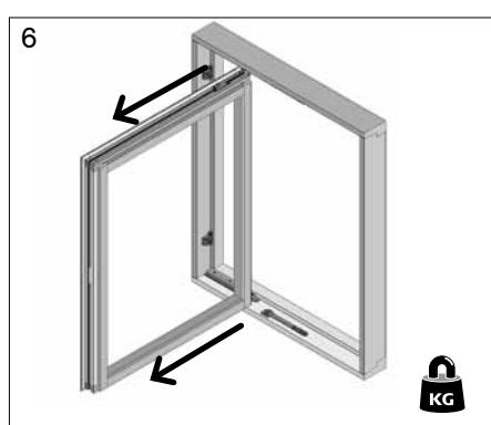
► **N.B. Remounting:** Make sure both locking plates are in the correct position, which is when only the locking signs are visible. If required the gliding rails should be lubricated with teflon-based lubricating oil (Never all-round lubricating oil!)
