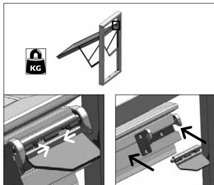
► **Support the sash and set the gliders free:** Squeeze the pointed screws towards each other with pointed pliers and free the sash from the frame.
