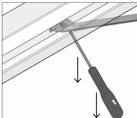
► **Dismounting:** Open the casement door ( $90^\circ$ ). Use a screwdriver to unclick the brake arm.
