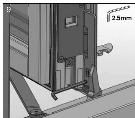
► **Height adjusting in the bottom hinge.** Open the window to maximum position. Take out the allen keys from the hinge side of the sash. First loosen the set screw placed horizontally at the hinge (9). Adjust the sash up or down by turning the set screw placed vertical at the bottom of the hinge (10). After adjusting tighten the set screw placed horizontally at the hinge (9).
