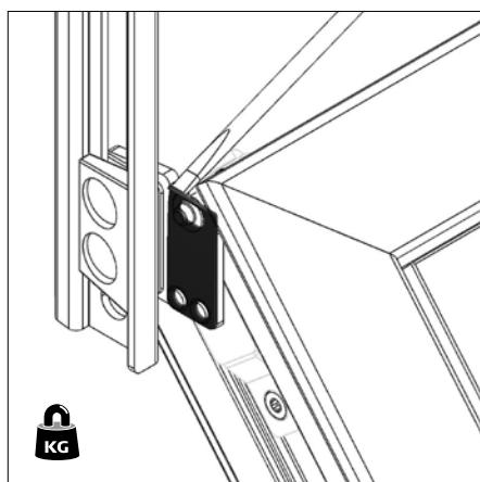
► Support the sash while dismounting the sash bracket (both sides), using a screwdriver to unclick them. The sash and frame is now separated.
