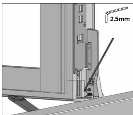
► After adjusting tighten the set screw placed horizontally at the hinge.
