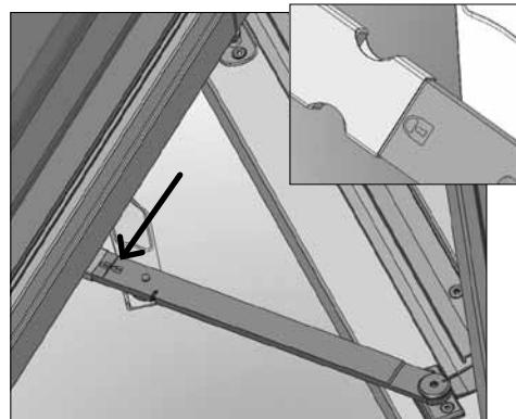
► **N.B. Remounting:** Make sure both locking plates are in the correct position, which is when only the locking signs are visible. If required the gliding rails should be lubricated with teflon-based lubricating oil (Never all-round lubricating oil!)
