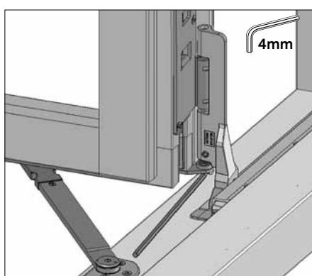
► Adjust the sash up or down by turning the set screw placed vertical at the bottom of the hinge.
