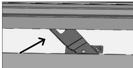
► **Dismounting:** Open the sash until the safety restrictor is activated. Pull back the sash slightly and detach the restrictor.
