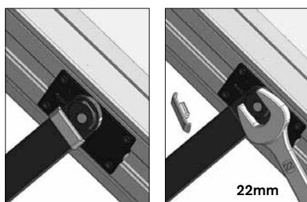
► **Height adjusting:** With a 22mm open-ended spanner turn the adjusting rivet on both sides of the sash as required. Eventually remove the protection plate while adjusting.
