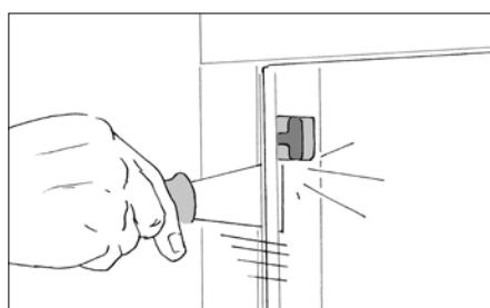
► **Move the putty knife until you locate the fixing clip nearest the corner.**
