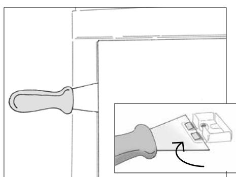
► **Release the fixing clip on the other side of the corner in the same way. Then pull the corner free. All clips must be released in the same way. Clips are positioned at app. every 40cm.**
