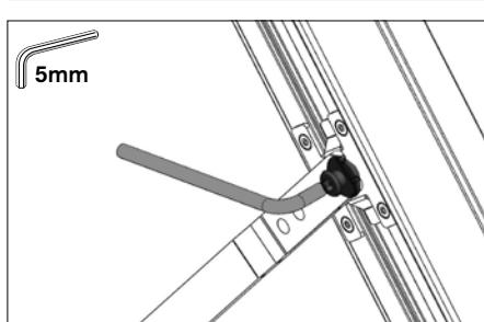
► **Height adjusting:** Turn the screw to adjust the sash up and down as required ( $90^\circ = 2 \text{ mm}$ ).
