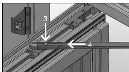
► Release the locking plates by holding down the lock button (3) while pushing the locking plate outwards (4) - top and bottom. Detach the guidearms from the rotating point at the sash using a screwdriver to unclick them, and turn the guide-arms away from the sash (5).
