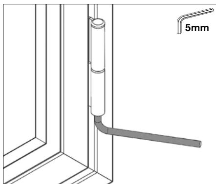
► **Height adjusting:** Turn the screw in the bottom hinge to adjust the sash up and down as required.
