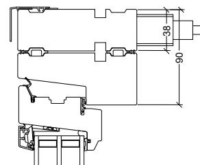
► Installed on 115mm mainframe
