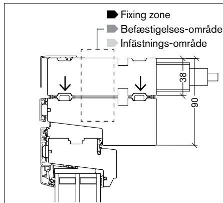
► The packer should be exactly the same length as the window unit.
