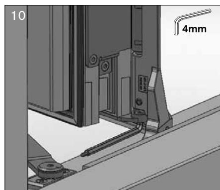
► **Adjust sideways:** Turn the adjustment screw in the sash mounting at the top and / or at the bottom of the frame.
