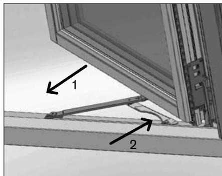
► **Dismounting:** Open the window and release an eventual safety restrictor. The sash will now lock in ventilation position, 30°, and cleaning position, fully reversed. To free these locks pull back the window slightly (1) and detach the restrictor (2).
