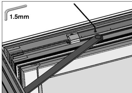
► **Adjusting the brake:** Open the casement door completely. Insert the key through the hole in the cover rail, then turn clockwise to tighten the friction brake.
