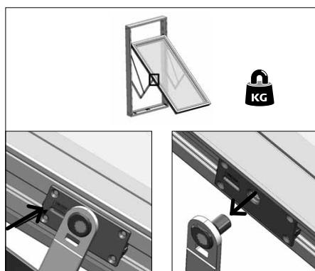
► **Continue supporting the sash and remove the sash mounting on both sides:** Place a screwdriver in the small hole next to the Unlock arrow and pull the screwdriver following the arrow. The sash mountings may now be released from the sash.
