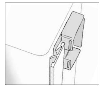
► **Pull back the putty knife slightly and move it in front of the clip. Push the knife forward to release the barb of the clip, then leave it in place.**
