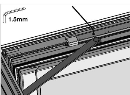
► **Adjusting the brake:** Open the window completely. Insert the key through the hole in the cover rail, then turn clockwise to tighten the friction brake.
