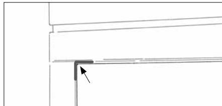
► **Dismounting the backboard:** Cut the sealant in all corners (2cm on both sides).
