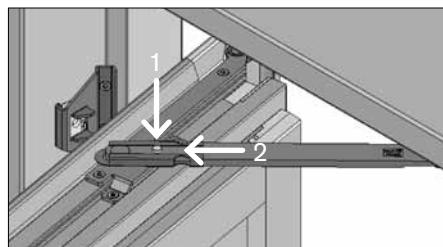
► **Dismounting:** Open the window to maximum position. Release the locking plates by holding down the lock button (1) while pushing the locking plate outwards (2) - top and bottom. Detach the guidearms from the rotating point at the sash and place the guidearms parallel to the frame pointing away from the guiderails (3).
