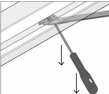
► **Dismounting:** Open the window ( $90^\circ$ ). Use a screwdriver to unclick the brake arm from the frame.
