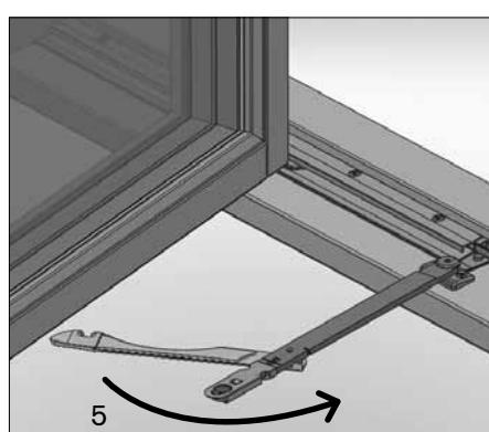
► Open the window to maximum position. Press the knobs at the end stops into the consoles (6) using a screwdriver and slide the hinges out of the rail (7). Slide the sash vertically out of the frame (8).
