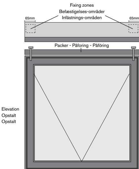
► **N.B.** don't screw through the vent itself. Fixing area is over the jambs.
