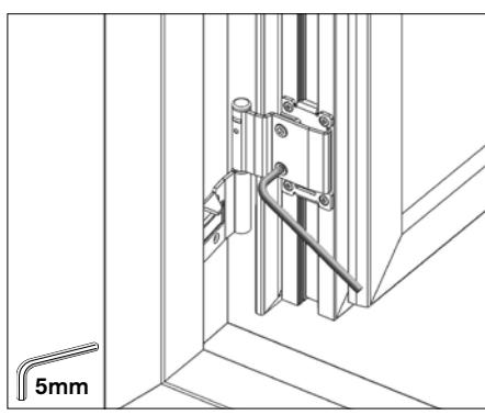
► **Adjust sideways:** Turn both screws per hinge to adjust the sash left and right as required. **N.B.** Adjust the screws equally in order not to twist the ironmongery. Turn each screw maximum  $\frac{1}{4}$  turn at a time.
